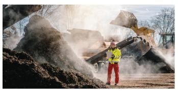
The material is placed in large piles, where microorganisms begin to break it down and heat up the piles to very high temperatures.
